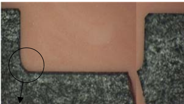
曲率半径 R:0.83mm R 止まり:0.30mm 継手側:225°
