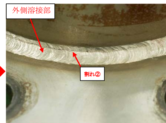
溶接部亀裂② ( 135^{\circ} )
